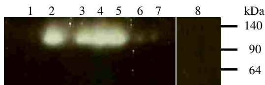
Fig. 1. Identification of BglA in C. cellulovorans and expression of rBglA. Lane 1: cellulosomal fraction of C. cellulovorans ; lane 2: non-cellulosomal extracellular fraction of C. cellulovorans ; lane 3: purified rBglA; lane 4: extracellular fraction of C. cellulovorans culture grown with cellobiose; lane 5: extracellular fraction of C. cellulovorans culture grown with ASC; lane 6: extracellular fraction of C. cellulovorans culture grown with xylobiose; lane 7: extracellular fraction of C. cellulovorans culture grown with xylan; lane 8: intracellular fraction of cellobiose grown C. cellulovorans cells. A 10 \mu l aliquot of the each fraction was applied to the polyacrylamide gel.
